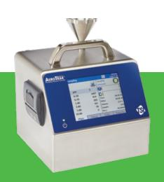
This particle counter can generate pass/fail reports for ISO 14644-1, EU GMP Annex 1, and FS209E, via the onboard printer and the supplied TrakPro Lite Secure download software. Multiple particle counter configurations can be conveniently stored and uploaded as needed. It can be used as a stand-alone particle counter or integrated into a facility monitoring system like TSI's FMS 5.
